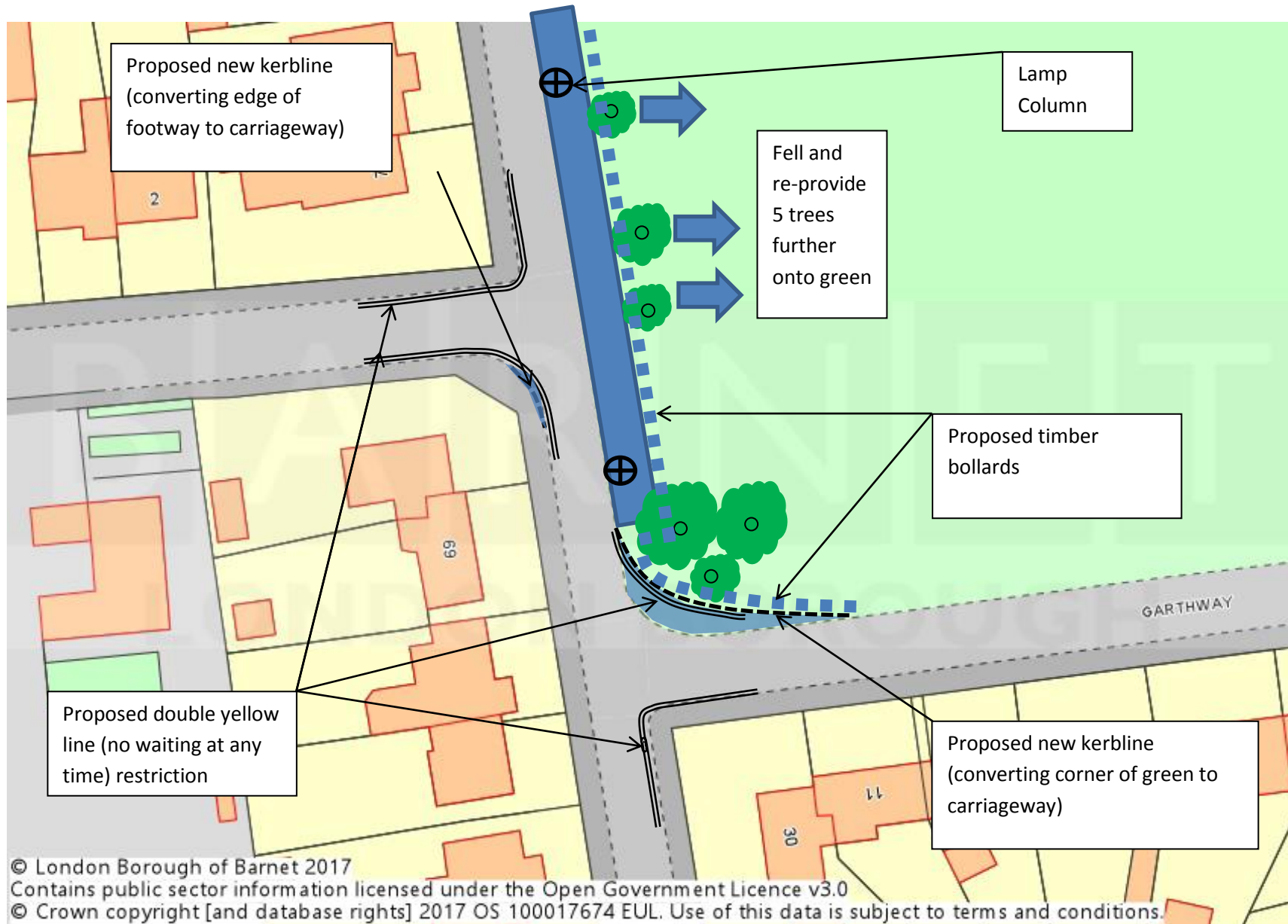
Inset B – Junction of Crescent Way and Garthway (Option 1). Parking restriction details and conversion to carriageway also relevant to option 2.
